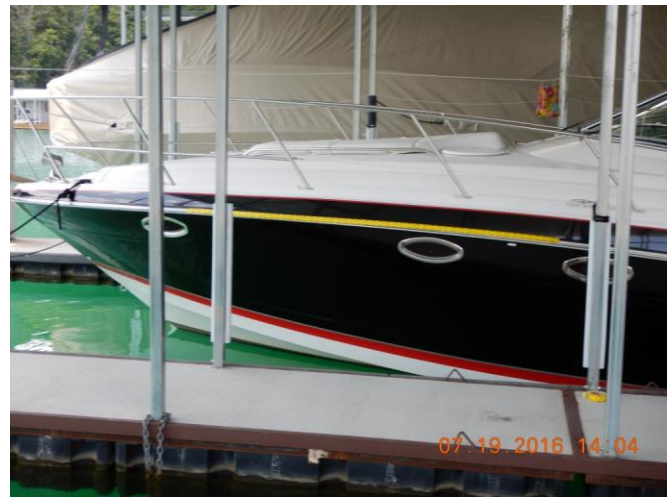
Figure 14 - Span of Damage to Gunwhale (Yellow Tape)
